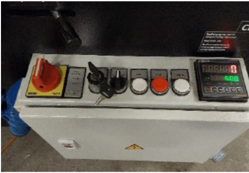
Control panel and mechanical coupling for automatic infeed and digital length measuring device
