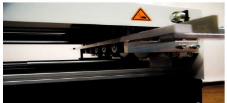
Secured drawer runner for manual access
