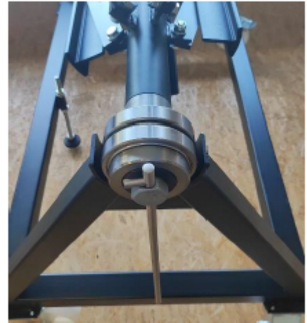
Spindle for adjustment of the expanding mandrel
