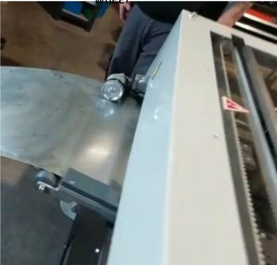
Sheet feeder with length measuring wheel
